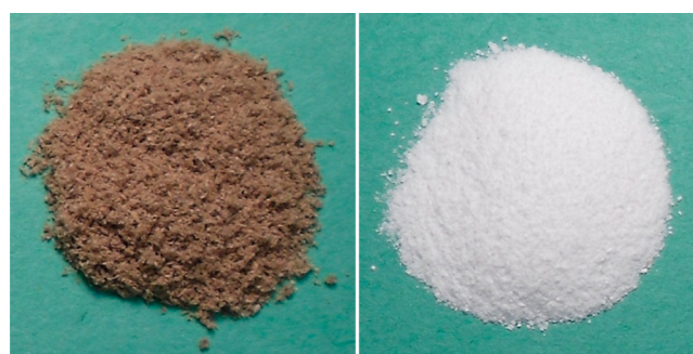
Figure 1. Regenerated LC from RHs before (left) and after bleaching (right).
